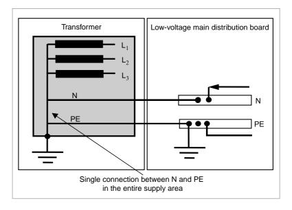
**Important prerequisite:** There is a separate N and PE bar in the low-voltage main distribution board. If not, it must be added.
