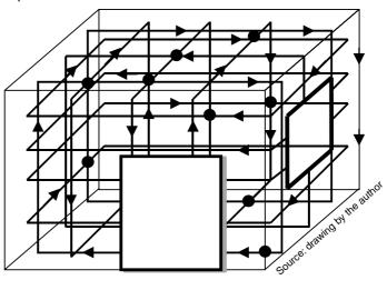
The figure shows the example of a current distribution system in a building as well as its earthing and equipotential bonding system. These currents are able to flow as soon as one PEN conductor is earthed at least twice.
