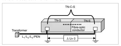
For such cases, VDE 0800 Part 2 stipulates the use of fibre-optic conductors.
