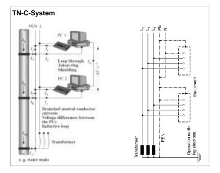
This installation is the cheapest minimum configuration that protects persons if installed skilfully and expertly. Nevertheless, this network configuration cannot by far offer protection for functions. As one PEN conductor is permitted in this network configuration, the neutral conductor currents inevitably flow through the PE conductor.
