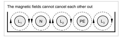
Values from practice: in an establishment, approximately 700 A rms flowed per subdistribution board and phase. In an office room directly behind, a magnetic field strength of 20  $\mu$  Tesla could still be measured at a distance of about two meters.
