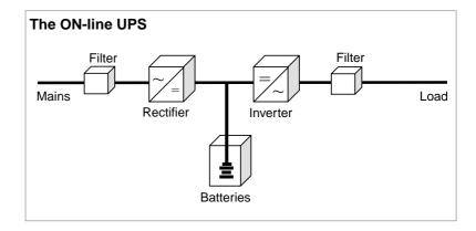
Operating principle: the mains voltage is filtered and rectified on the input end. On the one hand, the DC voltage charges a battery and, on the other hand, it serves as the input voltage for an inverter. This generates an AC voltage similar to a sine wave, which is then stepped up to an rms value of 230 V~. If the mains should fail, only charging of the batteries is suspended.
