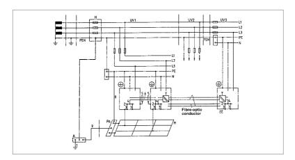
In practice, this means that the data cabling in the supply segments in which a clean TN-S network is installed with an unloaded PE can consist of copper data cable. Then, a fibre-optic cable must be used at the transition from one power supply segment to the other to avoid malfunctions and destruction.
