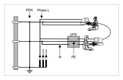
8 The standard electrical installation network configuration TN-C-S
