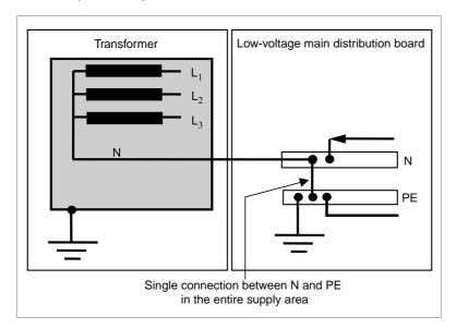
This variant is possible if the transformer and low-voltage main distribution board are not far removed.
