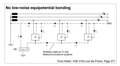
Neutral conductor currents in all earthed parts of an IT system
