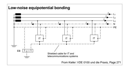
No neutral conductor currents in earthed parts of an IT system
