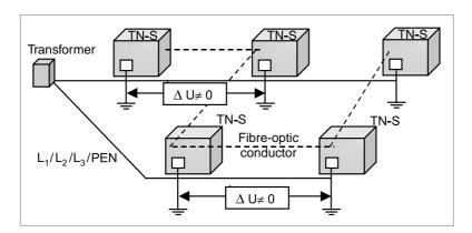
Fibre-optic conductors help to avoid problems
