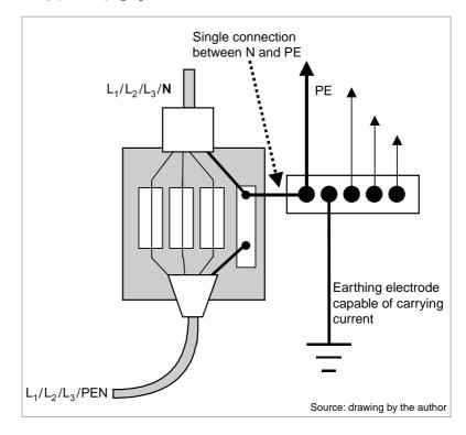
After the building transfer point, the PEN conductor is split into one N and one PE conductor and these are routed separately in the entire installation. The single connection between N and PE is at the PEN bar. There is also no connection via the meter positions and in the subsequent distribution boards, junction boxes, lamps and sockets.
